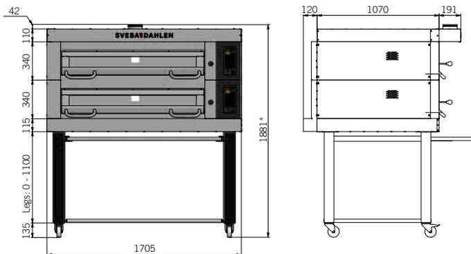
\* Example with two decks and leg height 800 mm
