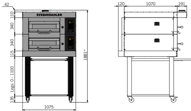
\* Example with two decks and leg height 800 mm
