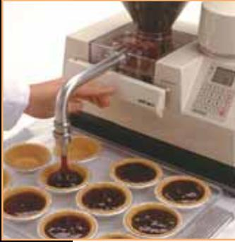
**PV-Series** The PV-Series power base gives the operator complete control over the speed at which a product is dispensed (which is not possible with the single speed power bases), the amount to be dispensed, the ability to adjust reversing of the pump after each cycle, automatic cycling and continuous dispensing. The ability to control all of these functions broadens the range of product applications.
