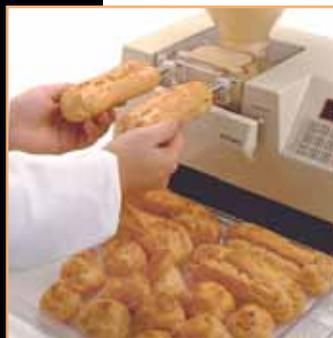
**PS-Series** The PS-Series power base offers the same reliability and maintenance-free design as the P-Series with the same controls and operating functions. The added benefit of the PS-Series power base is its 1/8 hp motor. The availability of higher power broadens the range of products that it can dispense. It is best suited for use with FS-Series and RP-Series filler units.
