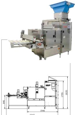
The Industrie Rex I is the classic entry-level model for high piece counts, as it can produce up to 24,000 pieces per hour. Due to the gentle dough processing with precise weight accuracy, not only the quantity but also the quality is correspondingly high.
