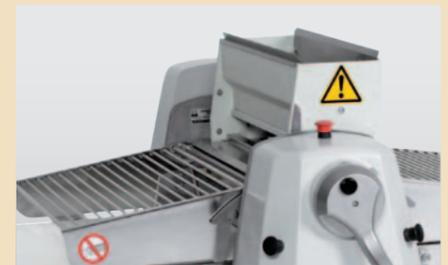
As an option, the Rondomat is available with a reversing lever. This is practical when you stand adjacent to the machine to get a better view of the dough band.
