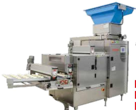
The Industrie Rex I is the classic entry-level model for high piece counts, as it can produce up to 24,000 pieces per hour. Due to the gentle dough processing with precise weight accuracy, not only the quantity but also the quality is correspondingly high.
